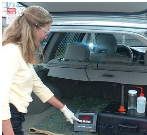
Figure 5 On-site use of an InfraCal TOG/TPH analyzer.
