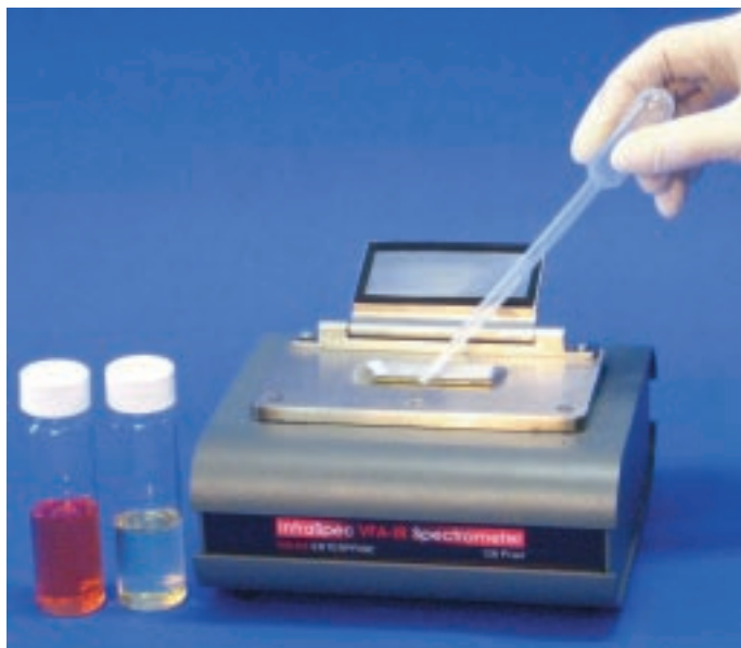
The InfraSpec VFA-12 Spectrometer used for the jet fuel study
